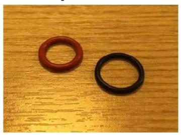
The washer on the left is for the Propulse G5 & PP17. The most obvious difference is that it is made of red rubber instead of black. It is also slightly thicker, and smaller in diameter.
